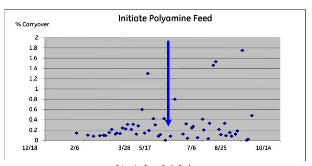
Polyamine Steam Purity Study % Carryover based on Steam/Boiler Water Sodium Levels
