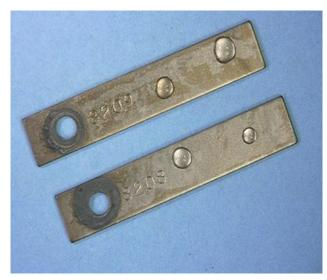
Polyamine can handle stressed conditions - Water beads on low carbon steel test coupons exposed for seven days to 10 ppm of polyamine product, 100 ppb of dissolved O<sub>2</sub> and 110°C (230°F) in deionized water. The average corrosion rate measured for them was 0.23 mpy (0.0060 mm/y).
